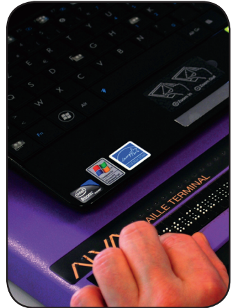
Braille terminal used for reading in Braille what is displayed on the screen. → Figure and caption
